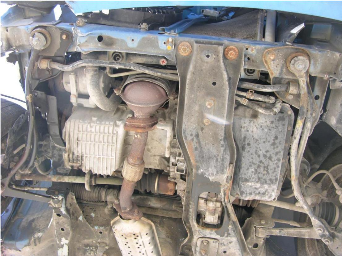
Figure 71. Undercarriage Damage, Test No. MGSMRH-2
