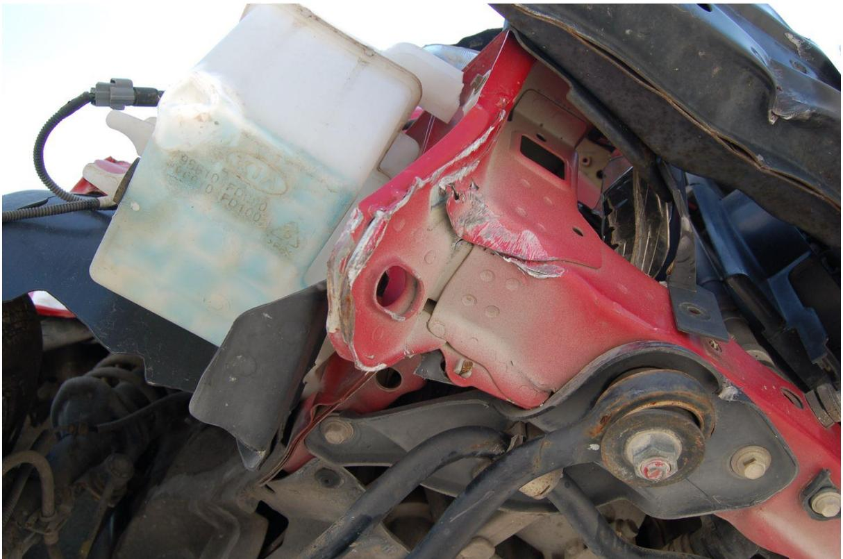
Figure 49. Undercarriage Damage, Test No. MGSMRH-1
