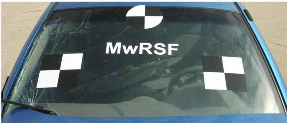
Figure 69. Vehicle Damage, Test No. MGSMRH-2
