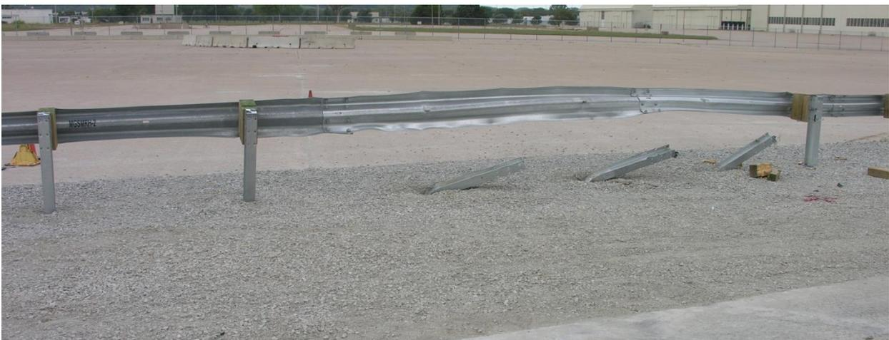
Figure 62. System Damage, Test No. MGSMRH-2
