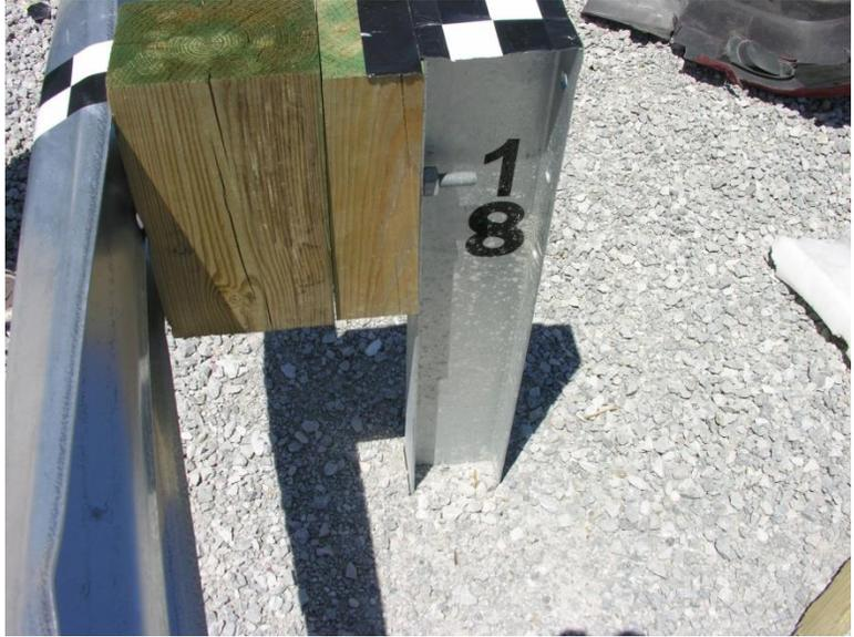
Figure 45. Post Nos. 17 and 18 Damage, Test No. MGSMRH-1
