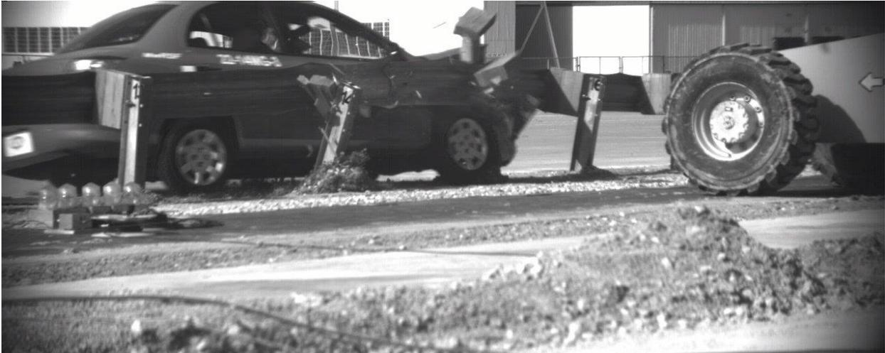
Figure 3. Test No. 2214MG-3, Wheel Snag
