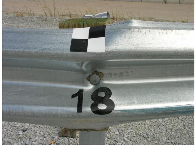
Figure 64. Post-To-Rail Bolt Hole Damage, Test No. MGSMRH-2
