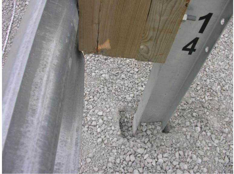
Figure 65. Post Damage, Test No. MGSMRH-2
