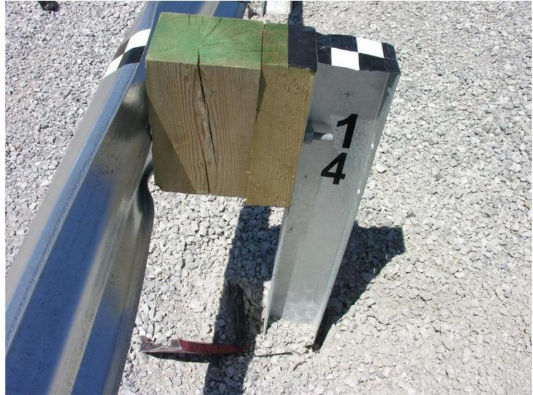
Figure 43. Post Nos. 13 and 14 Damage, Test No. MGSMRH-1
